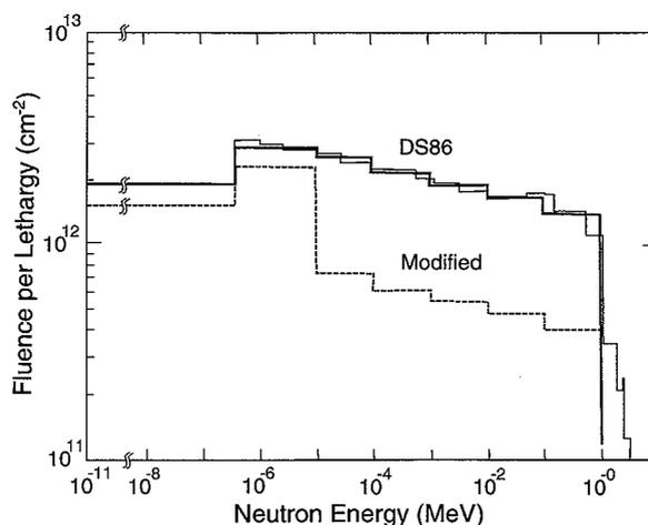
**Figure 2.** Neutron energy spectra at the location of the pillar. Thin solid line histogram indicates original energy-grouped fluence of DS86. Thick solid line histogram indicates reduced energy-grouped fluence used in the calculation. Dashed line histogram is an example of fluence modification to enable the calculated depth profile of  $^{152}\text{Eu}$  activity to reproduce the measured one.
