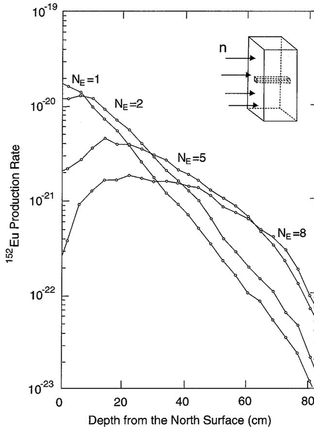
**Figure 3.** An example of calculated  $^{152}\text{Eu}$  production rate as a function of depth. Each depth point represents the cell's center position. Source neutrons are incoming normally to the north surface of the pillar. The four curves show the incident energy dependence of  $^{152}\text{Eu}$  production.
