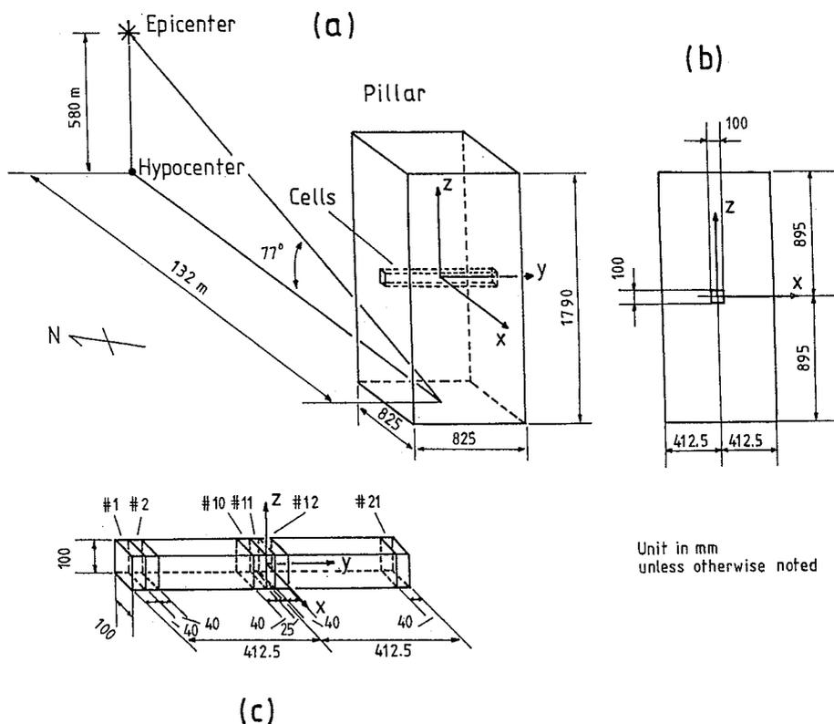
**Figure 1.** (a) Overview of the epicenter, hypocenter and the location and shape of the pillar, together with the coordinate system used in the calculation. (b) Side view of the pillar. (c) Size and numbering of the cells.
