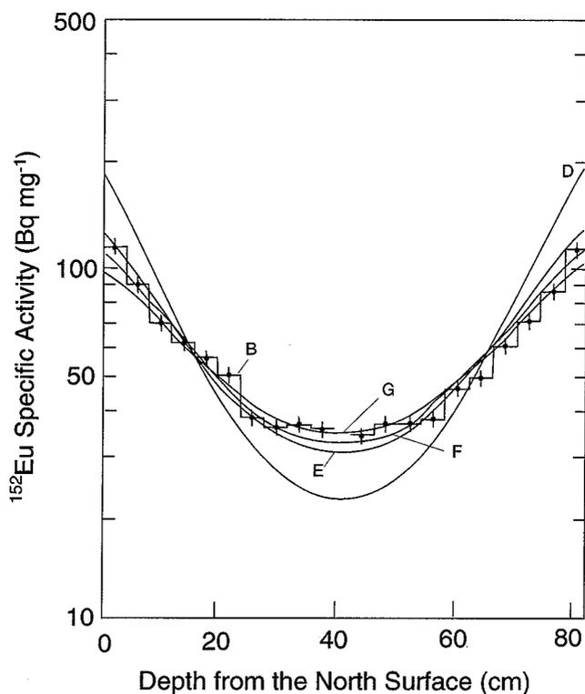
**Figure 5.** Depth profile of  $^{152}\text{Eu}$  specific activity (ATB) when the incident neutron spectrum was modified (Curves D, E, F and G). Curve F reproduces the measured profile (Histogram B) within the error of measured values. See the text for details.
