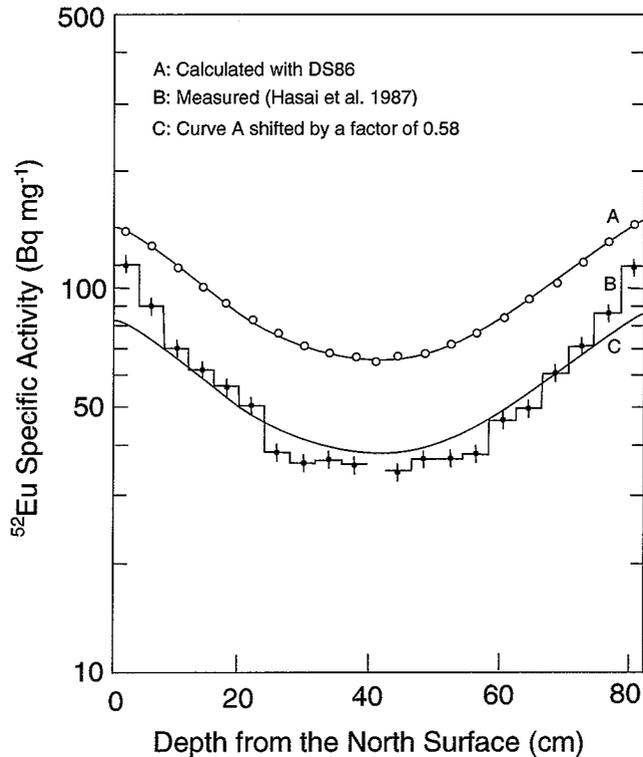
**Figure 4.** Calculated and measured depth profiles of  $^{152}\text{Eu}$  specific activity (ATB). Curve C is added to facilitate comparison.
