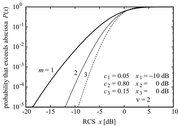
Fig. 6. Dependence of the probability on the number of pulses integrated.
