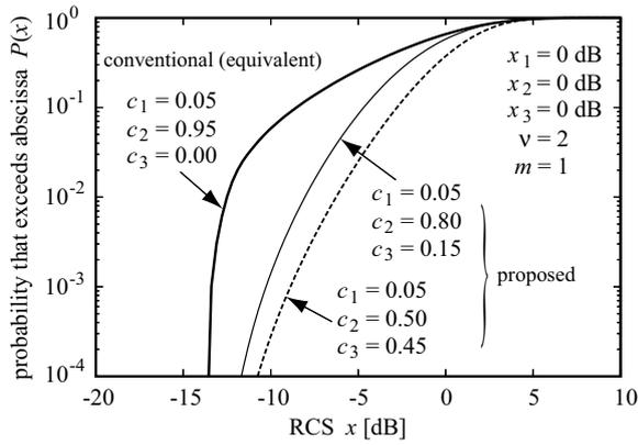
Fig. 3. Reception power distribution for various target-existence probabilities.
