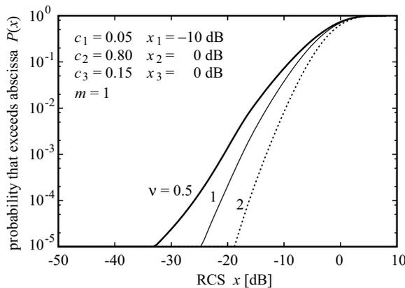
Fig. 7. Dependence of the probability on the shape parameter of the category 3 reflection object (single pulse detection).
