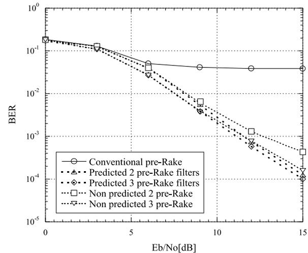
**Fig. 8** BER performance of the conventional pre-Rake system and the proposed systems based on predicted and non predicted channel impulse response in single user case using gold sequence with 4 paths and Doppler frequency of 200 Hz.
