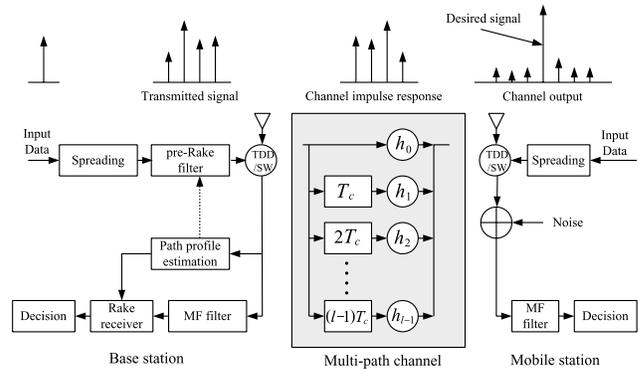
Fig. 1 The conventional pre-Rake system.
