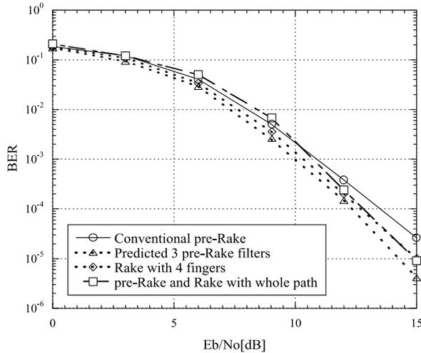
**Fig. 5** BER performance of the conventional pre-Rake system, Rake receiver with 4 fingers, conventional pre-Rake and Rake combiner with whole path fingers, and proposed systems based on predicted channel impulse response in single user case using gold sequence with 4 paths and Doppler frequency of 20 Hz.
