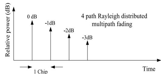
**Fig. 4** The channel model.
