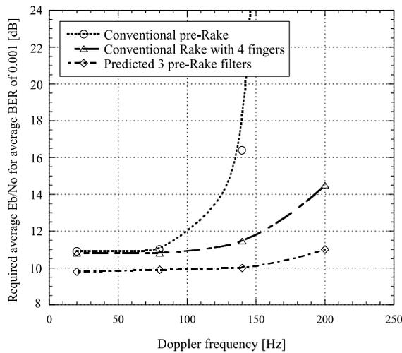
**Fig. 10** Required average  $E_b/N_0$  for satisfying average BER of  $10^{-3}$  of conventional pre-Rake system and our proposed system for various Doppler frequency and single user case.
