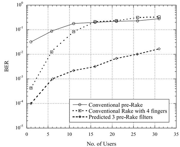
**Fig. 11** BER performance of the conventional pre-Rake system and our proposed systems using Walsh sequence versus the number of users for  $E_b/N_0 = 15$  dB, number of paths is 4, and Doppler frequency of 200 Hz.
