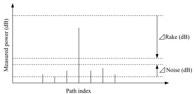
Fig. 2 The received signal path pattern using the pre-Rake filtering in the transmitter.
