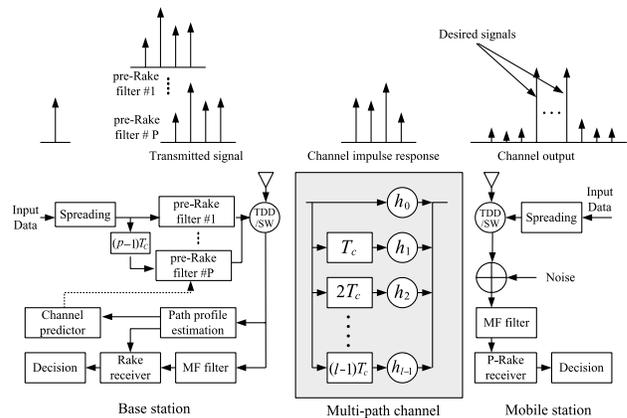
**Fig. 3** The proposed system using multiple pre-Rake filters in transmitter and a Rake combiner in receiver.
