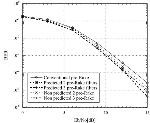
**Fig. 7** BER performance of the conventional pre-Rake system and the proposed systems based on predicted and non predicted channel impulse response in single user case using gold sequence with 4 paths and Doppler frequency of 20 Hz.
