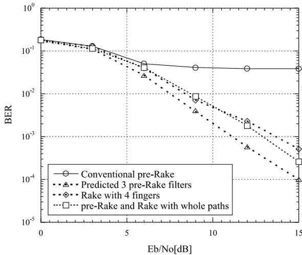
**Fig. 6** BER performance of the conventional pre-Rake system, Rake receiver with 4 fingers, conventional pre-Rake and Rake combiner with whole path fingers, and proposed systems based on predicted channel impulse response in single user case using gold sequence with 4 paths and Doppler frequency 200 Hz.
