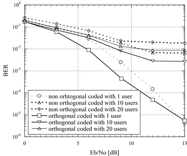
**Fig. 9** BER performance of orthogonal and non-orthogonal coded system for various user cases with predicted 3 pre-Rake filtering system and Doppler frequency of 20 Hz.
