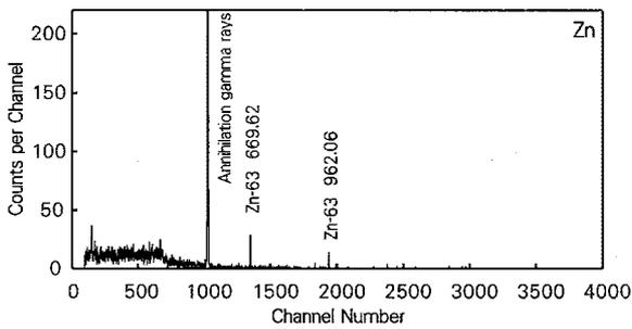
Fig.2 Gamma-ray spectrum for zinc foil. The measurement started 38 min after the end of the X-ray exposure, and lasted for 600 s.
