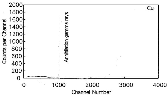
Fig.3 Gamma ray spectrum measured for copper foil. The measurement started 7 min after the end of the X-ray exposure, and lasted for 300 s.
