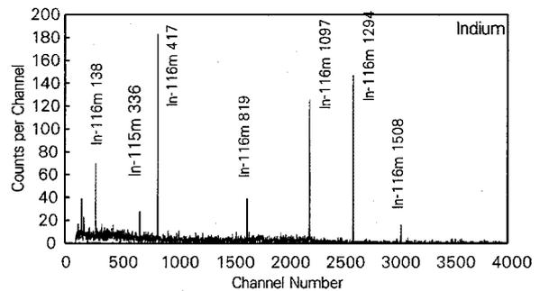
Fig.5 Gamma ray spectrum measured for indium foil. The measurement started 40 min after the end of the X-ray exposure, and lasted for 600 s.
