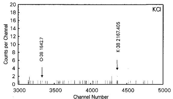
Fig.6 Gamma ray spectrum measured for potassium chloride. The measurement started 5 min after the end of the X-ray exposure, and lasted for 5 min.
