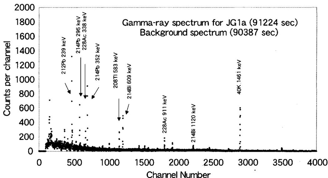
**Figure 2** Gamma-ray spectrum for 25 g of GSJ reference sample (JG1a). Background spectrum was measured without any sample and was subtracted from the spectrum for JG1a after adjusting the difference in elapsed times for measurements.
