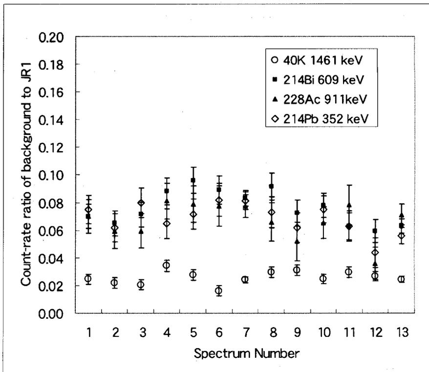
**Figure 4** Ratios of gamma-ray count-rate in background to that of the JR1 reference sample. Count rates of full energy peaks were obtained from 13 background spectra and a spectrum for the JR1 reference rock sample. The vertical axis indicates the ratio of background count rate to that of the JR1 spectrum.
