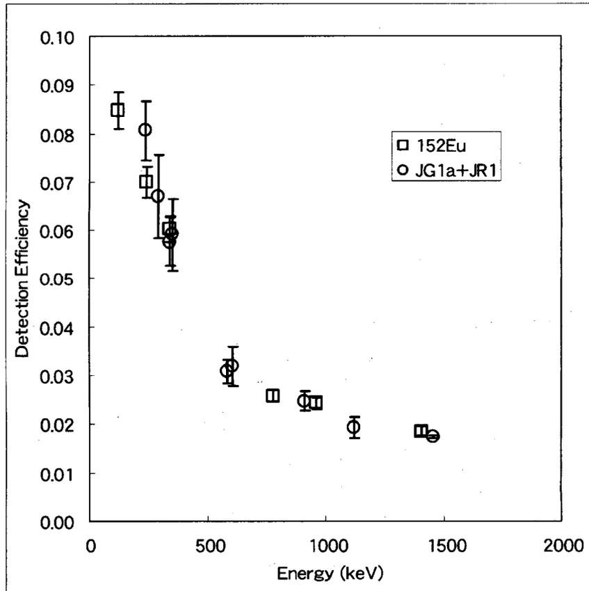
**Figure 3** The detection efficiencies examined by the GSJ reference rock samples (open circles: JG1a + JR1), and estimated by the  $^{152}\text{Eu}$  point-like standard source (open squares:  $^{152}\text{Eu}$ ).
